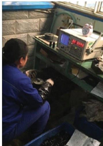
LOAD PIN CRACK DETECTION AND INSPECTION
